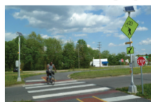
User-activated flashing sign (Rectangular Rapid Flashing Beacon)
